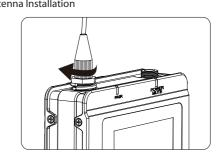
\* When installed, the TX antenna is away from the human body (belt clip), which helps to improve the transmission distance.
