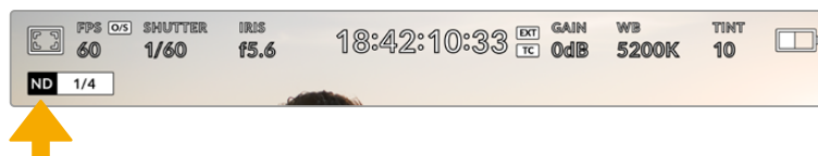
ND filter setting indicator on your URSA Broadcast
