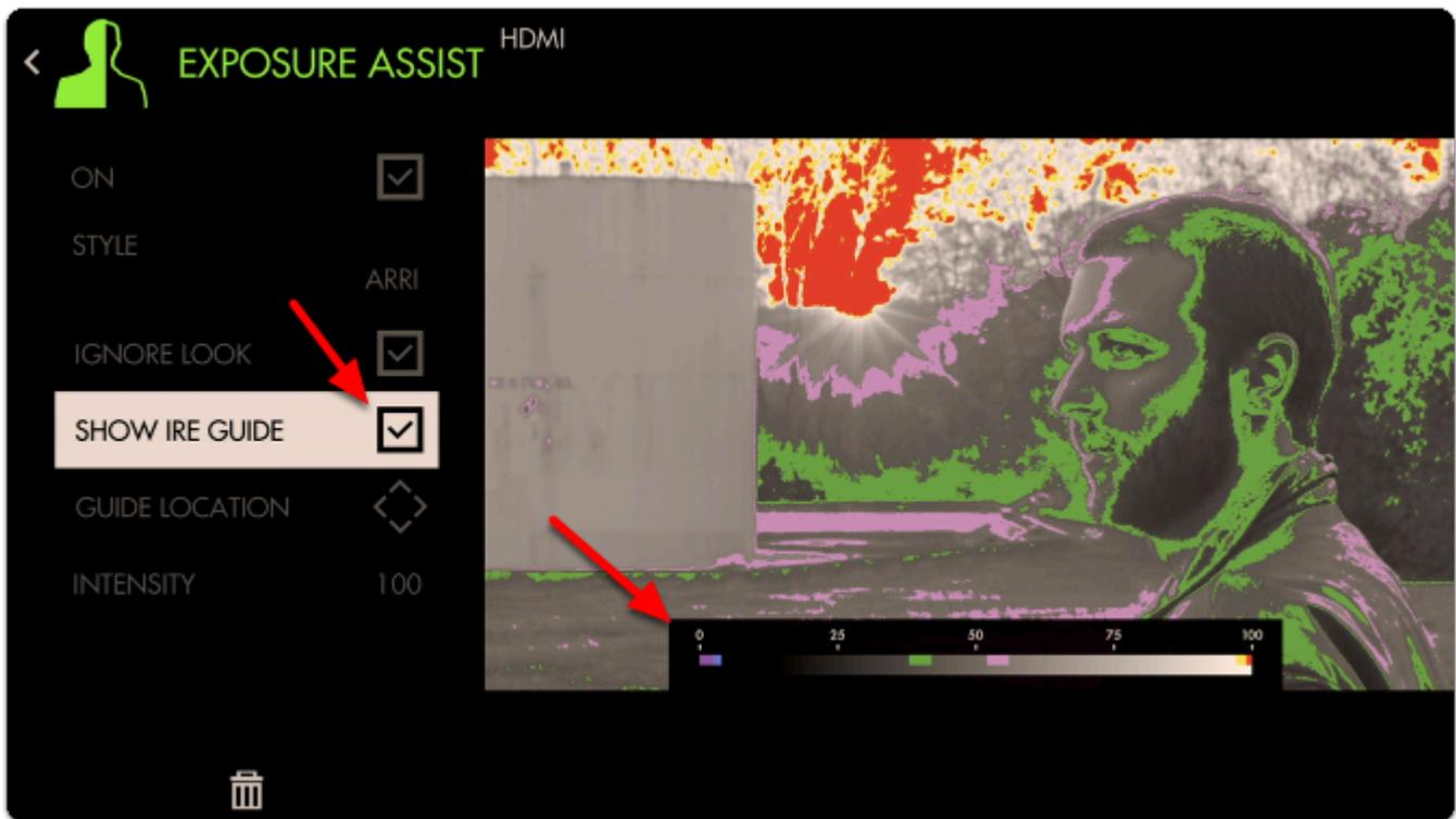
Exposure values near the **50%** mark on the scale will generally provide the most **natural result** on **human skin**. With the **Arri scale** this means the **pink** and **green** bands provide a great guide as the **upper** and **lower** range for exposing faces.
