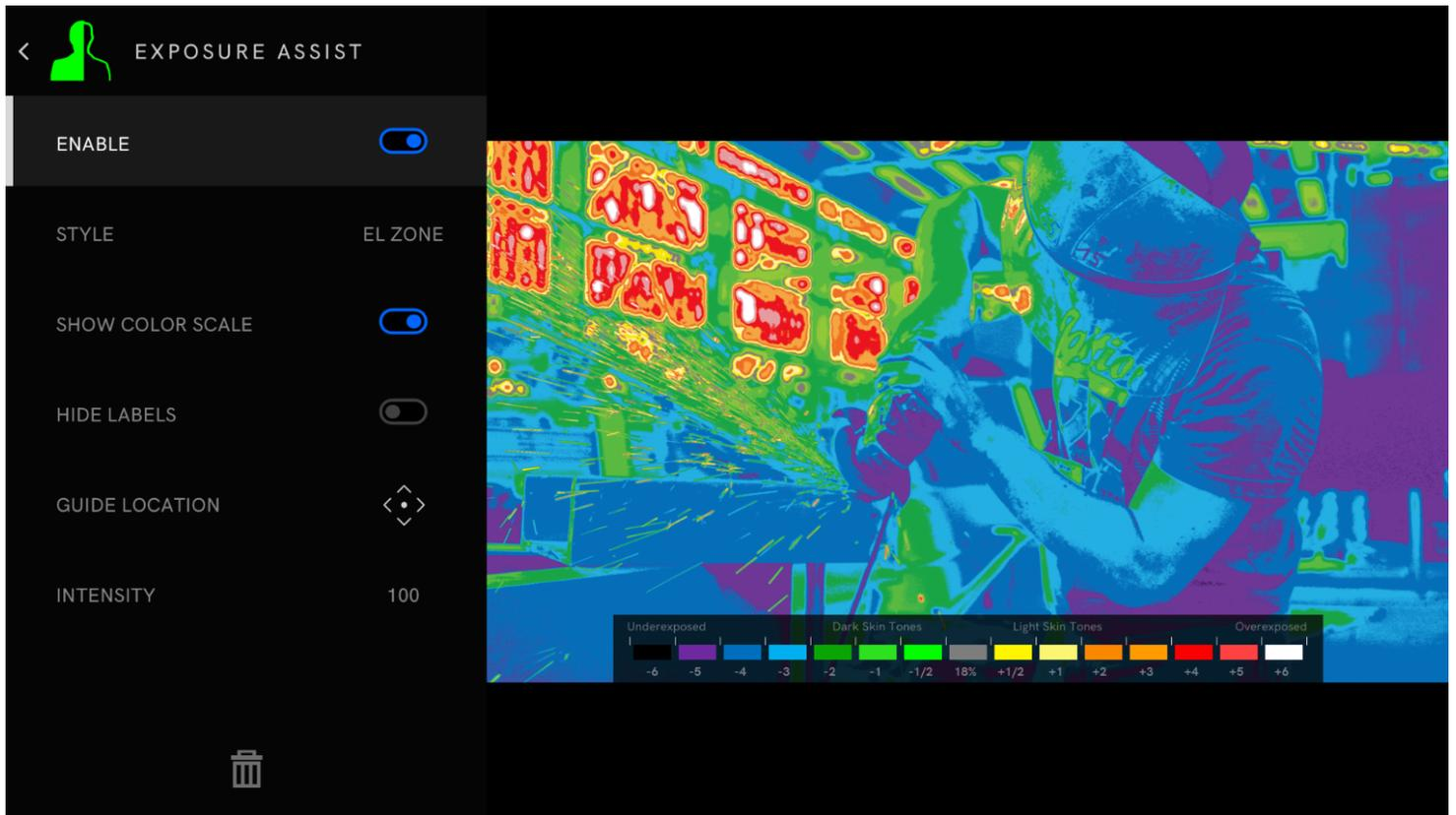
EL Zone is a stop-based exposure map tool—developed in collaboration with legendary cinematographer Ed Lachman, ASC that works like a virtual spot meter, replacing IRE exposure values with stops. Sensor data from the camera provides a reference point, and a false color represents each stop above and below 18% gray, allowing for easier, more intuitive on-set communication.
