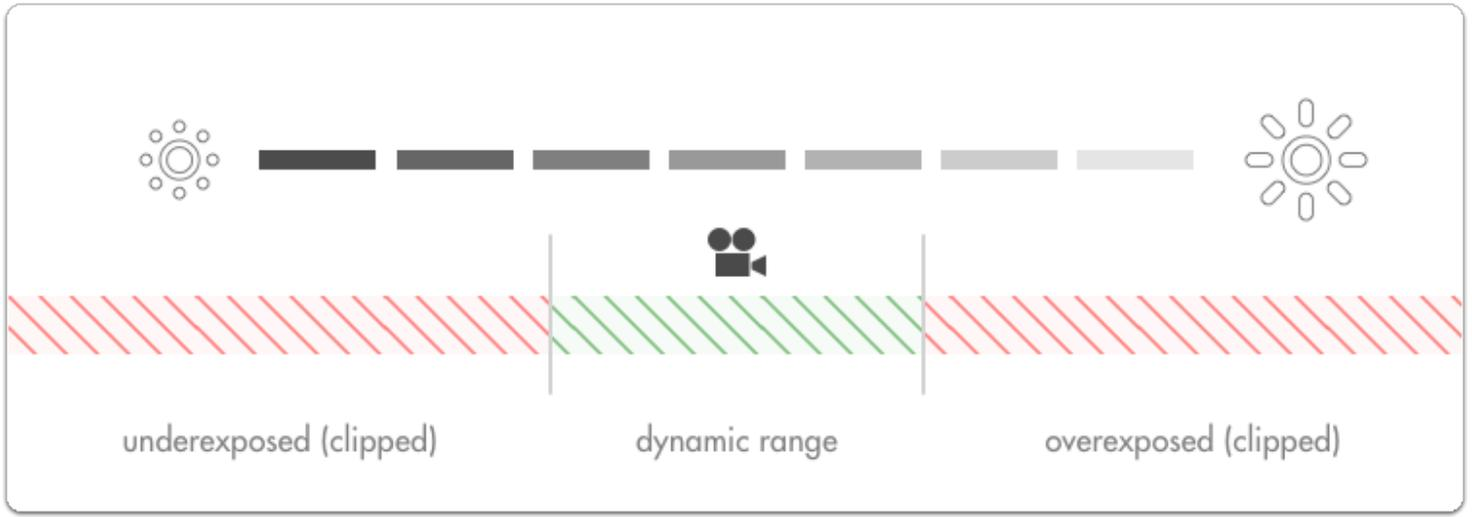
Adjusting **exposure** will shift the **dynamic range** to capture brighter or darker detail in order to accommodate the most important aspects of the image. Anything outside the **dynamic range** gets **clipped**, meaning a badly placed exposure is **wasting the camera's potential**.
