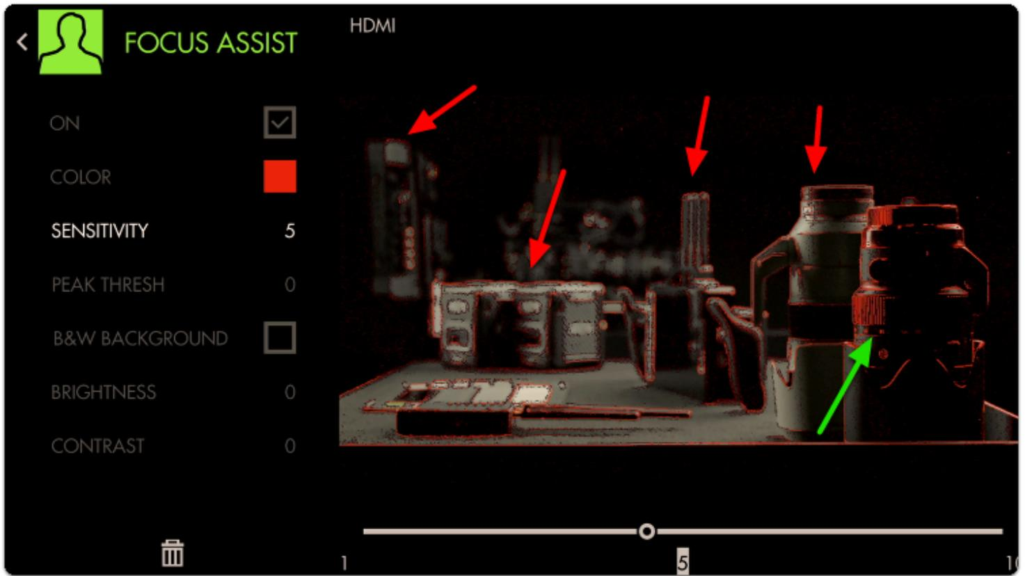
Notice how we are picking up many edges that are **not in focus** in addition to the areas that **are in focus**. **Increase** the next slider labeled '**Peak Thresh**' to help eliminate the false positives.
