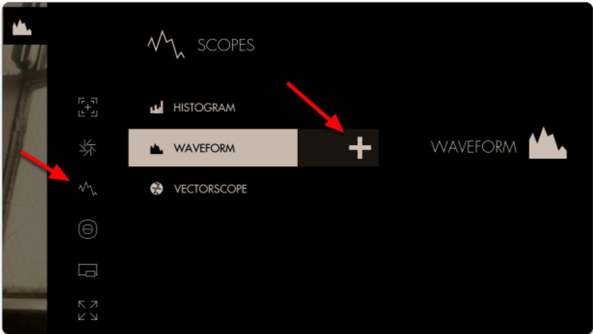
Once added you can **edit the settings** by **navigating right** when 'Waveform' is highlighted.
