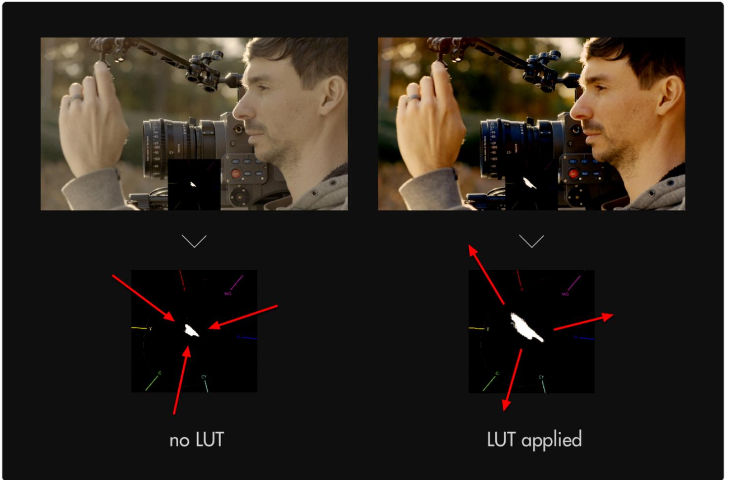
💡 The Vectorscope uses the same layout as a **color wheel** and therefore principles of **color theory** apply - for example we can achieve **complimentary** colors by ensuring our scene plots to the graph on **exactly opposing sides**. Perhaps the most common example of this is the famous/infamous 'teal/orange' look popularized in Hollywood where skin is orange and nearly everything else gets colorized as teal.
