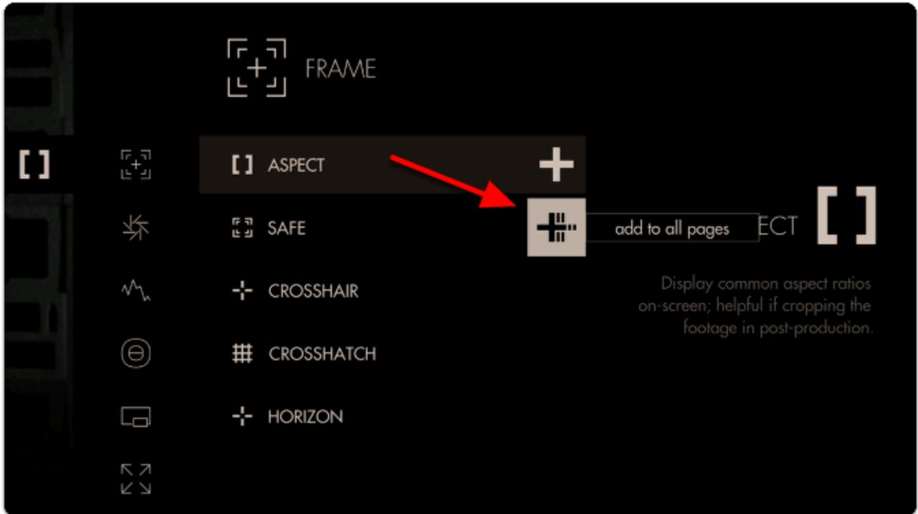
This will ensure you are able to **view this tool on every page** of the monitor, and any edits to it are made **globally**. Any tool can be added to all pages, including scaling adjustments and Look (3D LUT) files.
