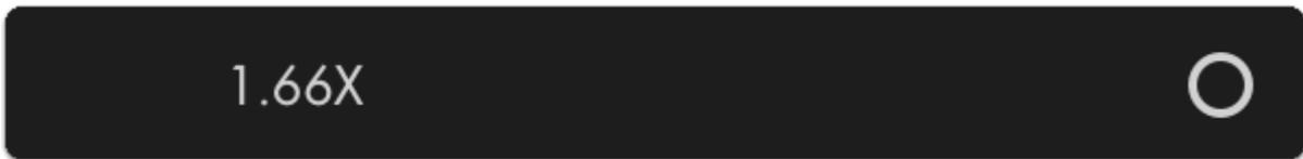
Use to de-squeeze anamorphic footage using lenses or adapters with a 1.66X squeeze factor.
