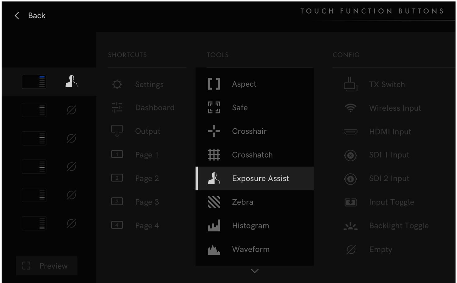
Notable configurations for Touch Function Buttons include Backlight Toggle, Backlight Custom, Input Select, and 4K TX Switch. Having different inputs on Touch Function Buttons allows the user to quickly switch sources, without having to navigate to the Monitor Settings menu.
