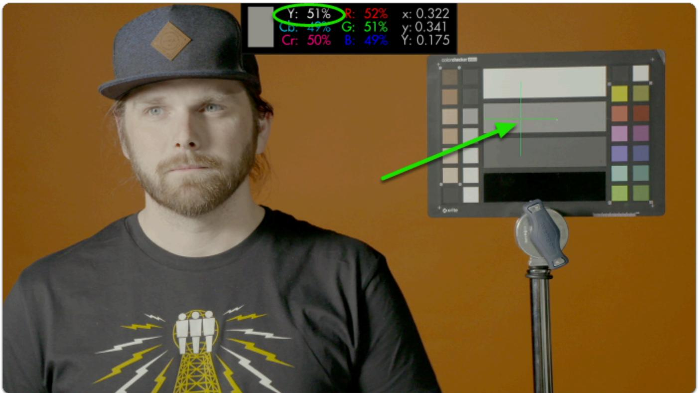
This particular color chip has been designed to read as 'middle grey'. Look for the 'Y' (luma/brightness) percentage and roll exposure until it reads **near 50%**.
