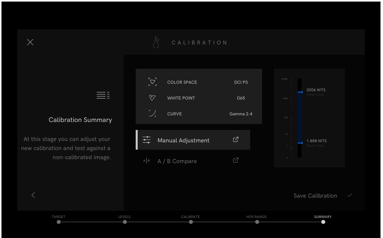
9. Your new calibration profile will automatically be applied and listed as **Custom Calibration** in the Calibration settings. You can toggle between **Custom Calibration** and **Factory Calibration** at any time.
