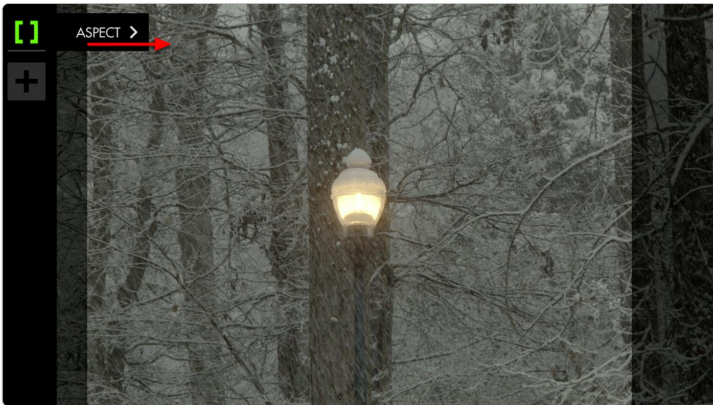
The **default** setting is for previewing a **4:3** aspect ratio for older TVs. Select '**Ratio**' and change it to **2:39** to see the black bars switch to a horizontal configuration.
