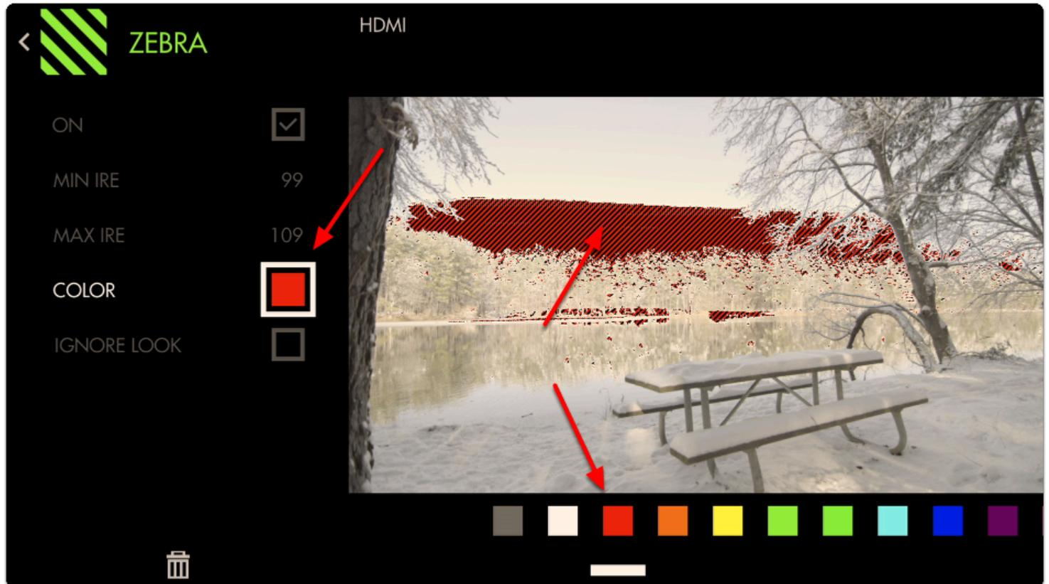
At this stage we can roll **exposure down**, add an **ND filter**, **decrease ISO** or **increase shutter speed** to **darken** the image until the zebra pattern is no longer visible to get **highlight detail back**.
