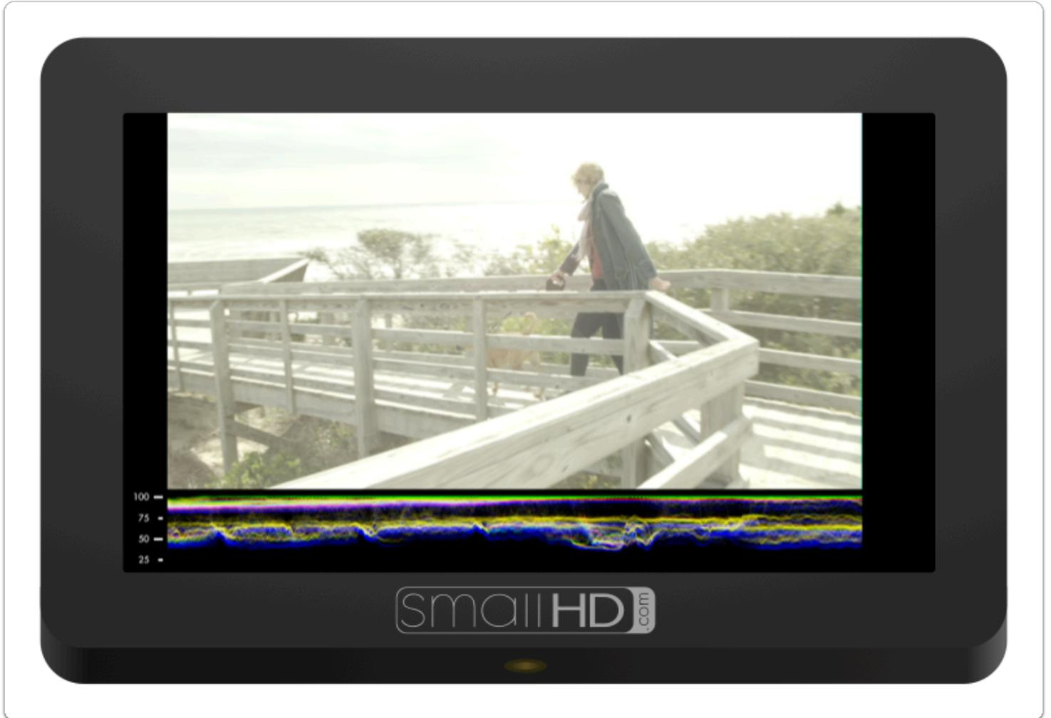
Waveform plots the value of the entire image onto a graph that physically matches it from left-to-right, meaning if you see an area that's too bright on the left side of the image, it will create a 'peak' on the left side of the waveform graph. It also has other benefits by way of RGB & RGB Parade modes. [Click to learn more about the Waveform.](#)
