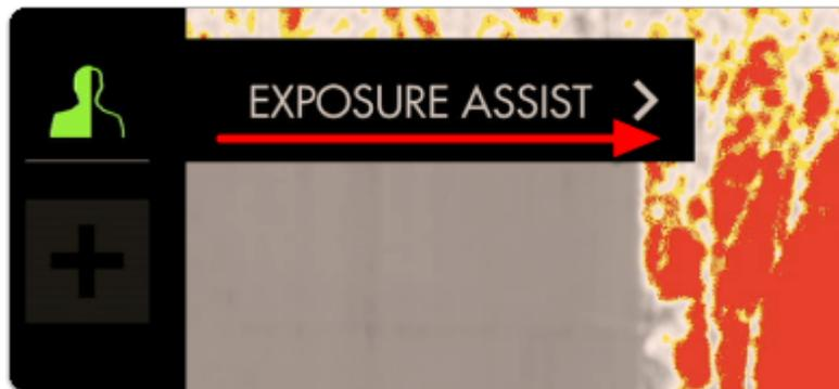
By default the **Arri False Color** scale is used which is a great place to start. Another scale is the **Spectrum** False color, which is a gradient of color from Pink-Blue-Green-Yellow-Red. This is easily seen on the Guide bar.
