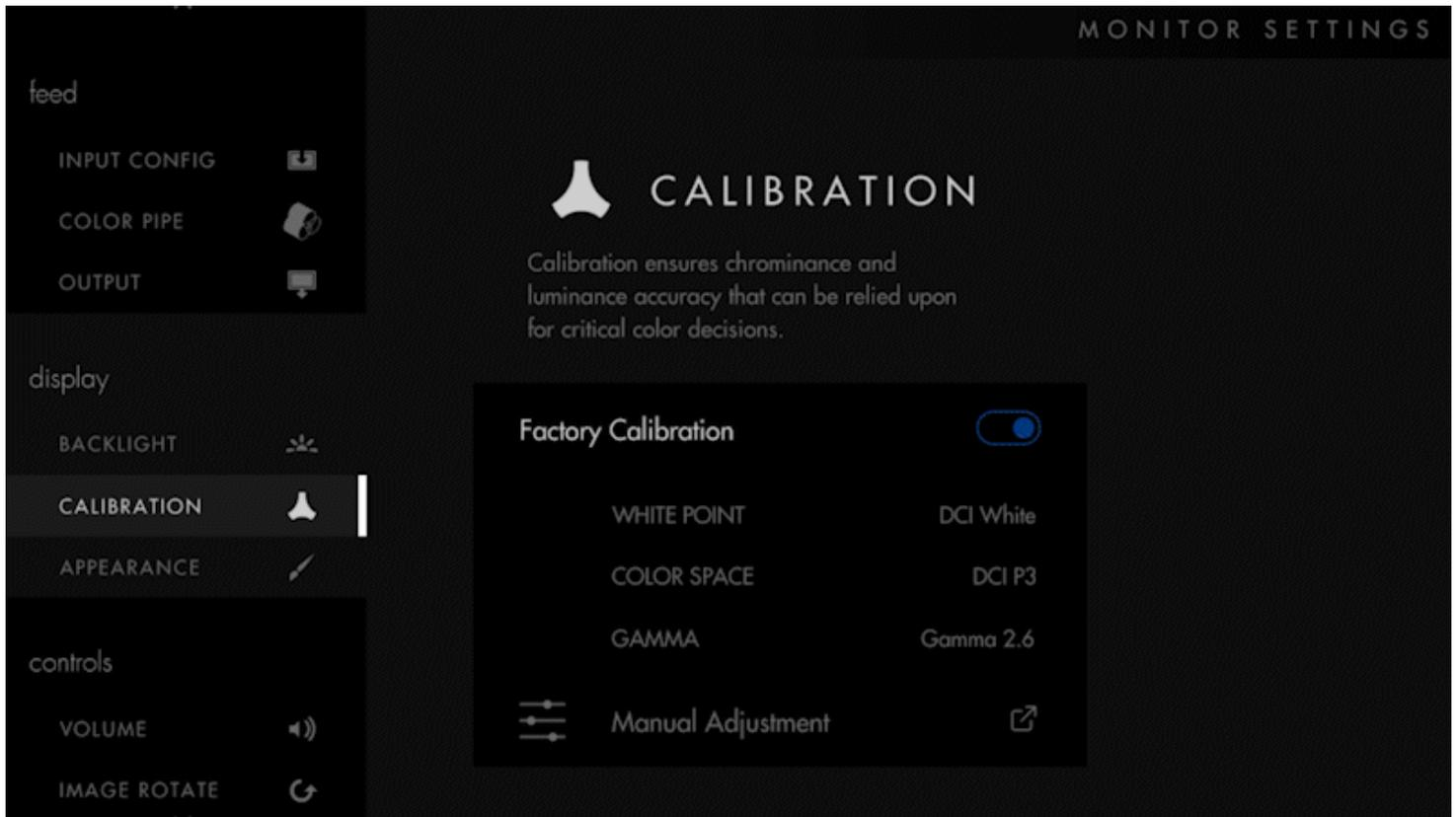
After clicking through the introduction, you will choose your calibration target. For non-HDR monitors, SDR - REC709 will be the recommended calibration. Select your calibration target and in the next screen, select Accept Calibration Target.
