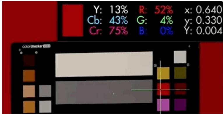
**Color Picker** samples color/value information from a **single pixel** to give a precise readout of a specific location. Great for **matching** multiple cameras or getting **consistent exposure** in changeable lighting conditions by sampling from a color chart or an actor/subject's face.
