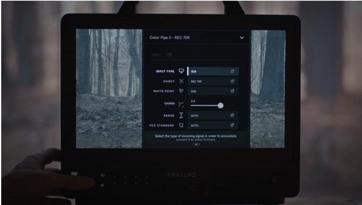
**INPUT TYPE** will be what signals the Monitor accepts. The default is **SDR**.
