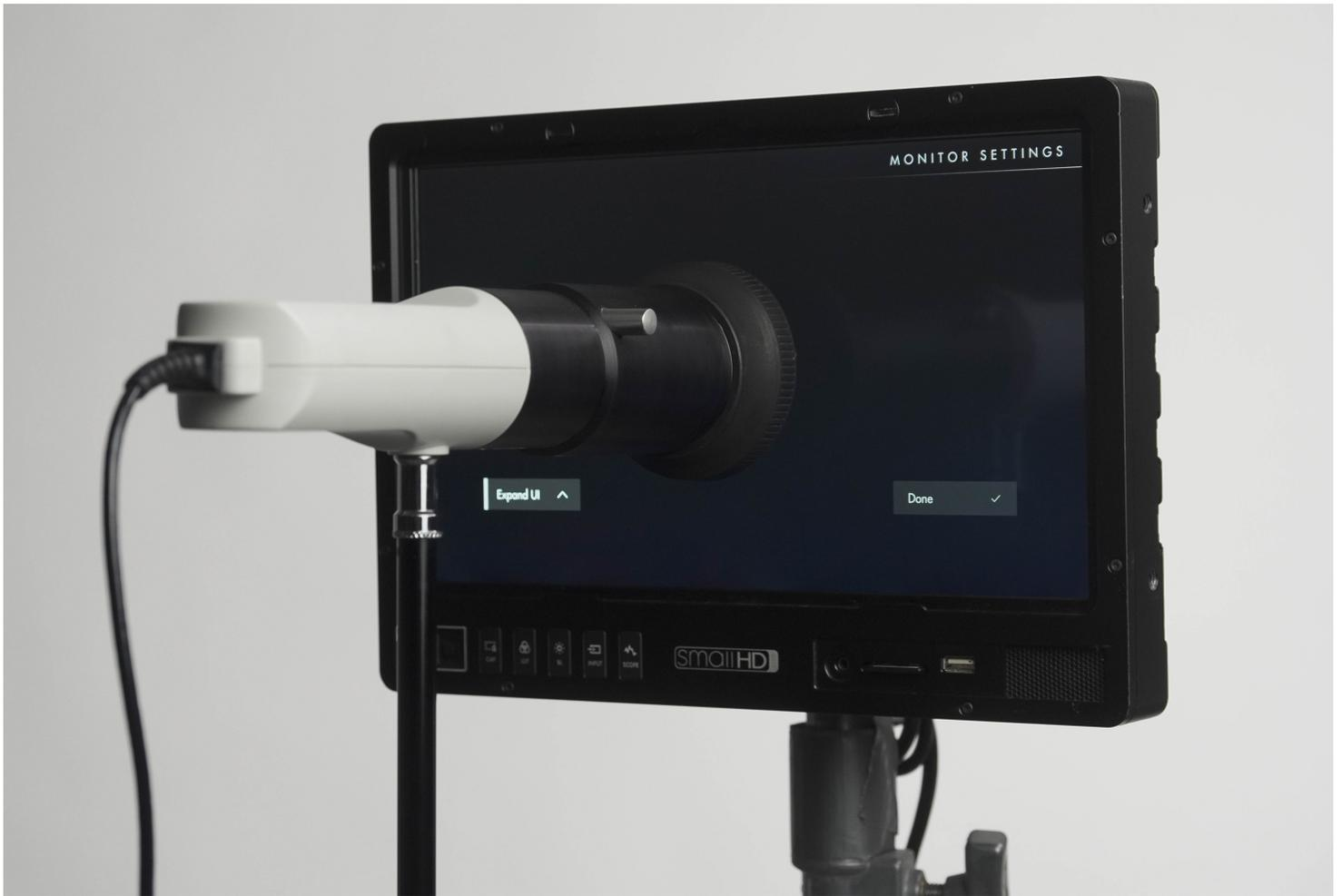
Follow the DisplayCal instructions, making sure that you have the correct monitor and probe selected. Also make sure that your calibration settings match the calibration target. We are not affiliated with DisplayCal so please refer to the documentation and support from DisplayCal for operating the software.
