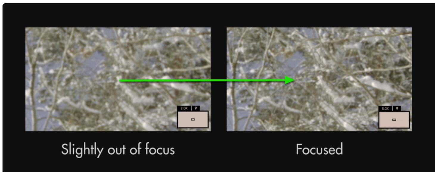
Though a minor adjustment, this has **increased the effective resolution** of the entire image.
