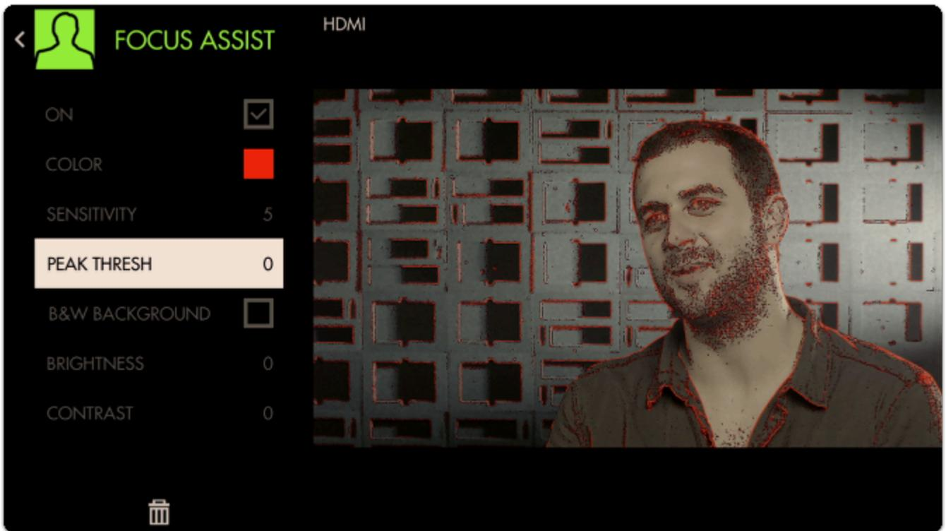
Bringing **Peak Threshold** up to around 30 does a better job of causing **only in-focus areas to activate the filter** but this is ultimately a balance that may need tweaking depending on the camera/shot.
