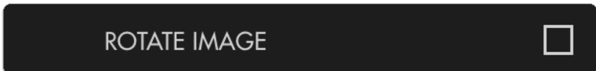
This will rotate the displayed image 180° bypassing any automatic functionality
