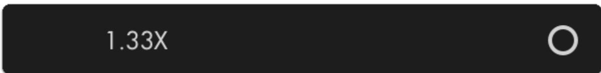
Use to de-squeeze anamorphic footage using lenses or adapters with a 1.33X squeeze factor.
