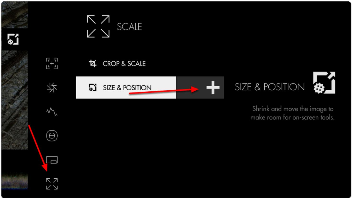
Once added you can **edit** the settings by **navigating right** when '**Size & Position**' is highlighted. Navigate to **SIZE** and adjust it from **100** to **75**- you will notice the image scaling from its' center point.
