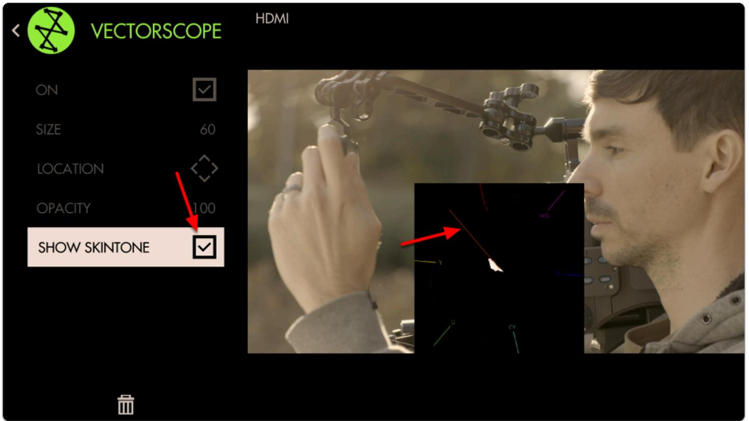
Because the **entire image** is being plotted to the graph all at once, we can check the status of individual areas by using **Pixel Zoom** in combination with the **Vectorscope** for **spot meter** functionality!
