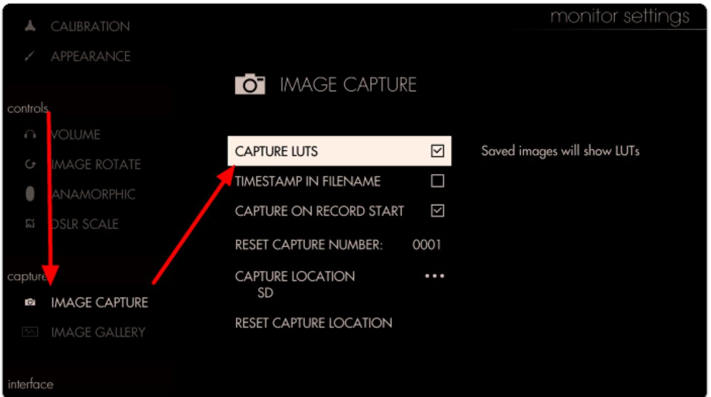
Flip back over to the page with **Image Capture** applied so that we can take a snapshot.
