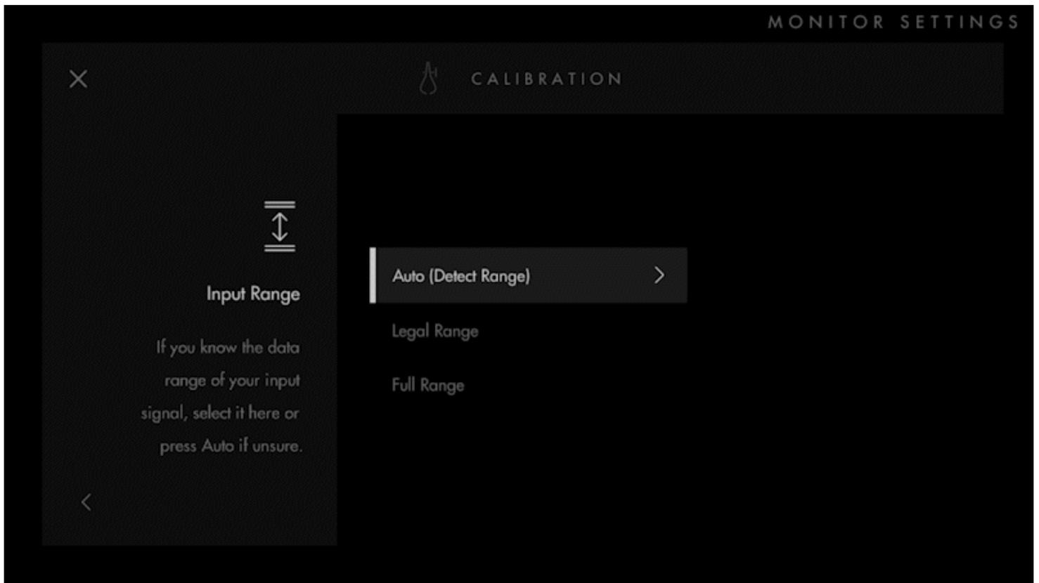
Next you will Calibrate. Select Next and you will be brought to a calibration UI that will display the feed from your computer with no calibration applied, so your probe can start measuring.
