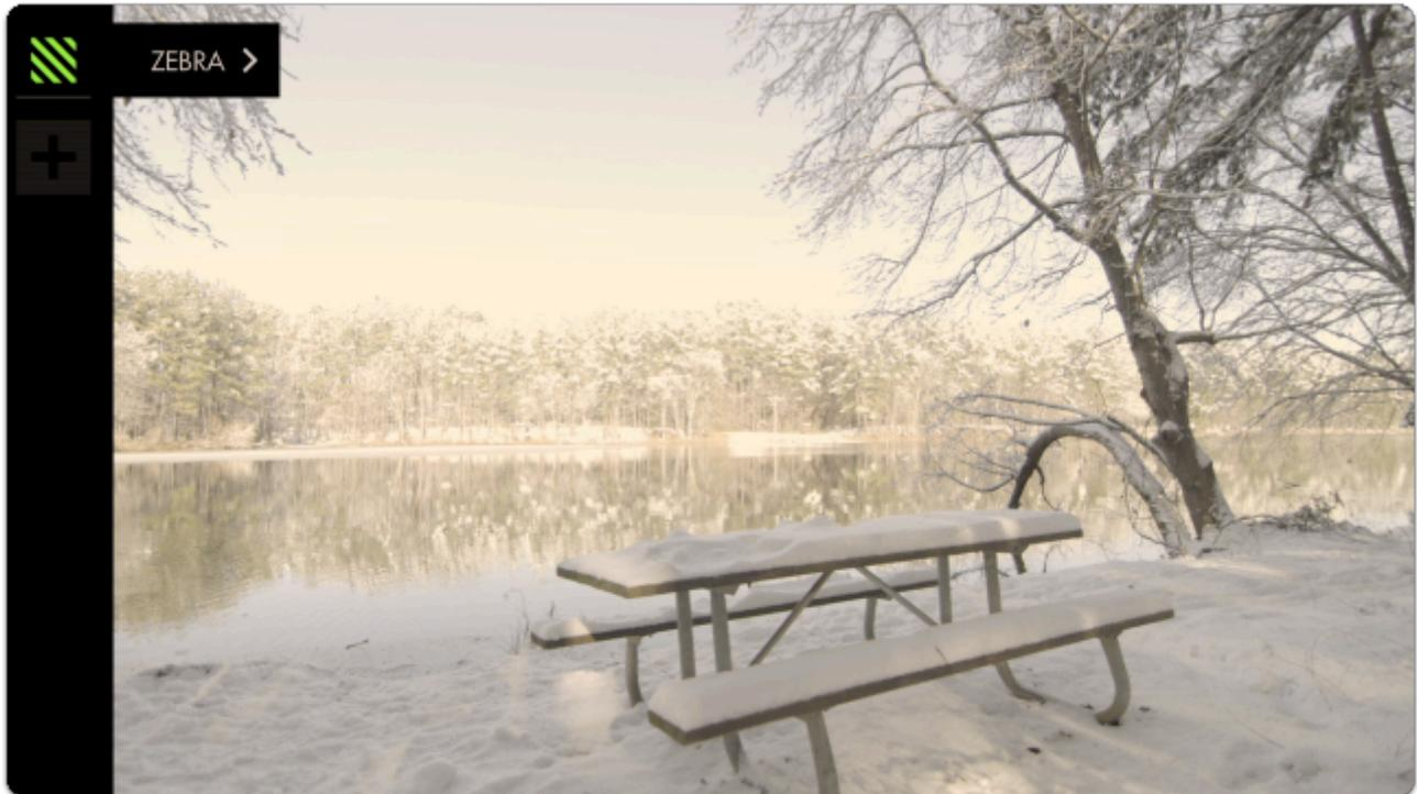
Because our camera **places its overexposure limit below 100%** or 100 IRE (quite common when shooting in log/flat gammas) **we need to adjust the minimum IRE** until the Zebra is activated.
