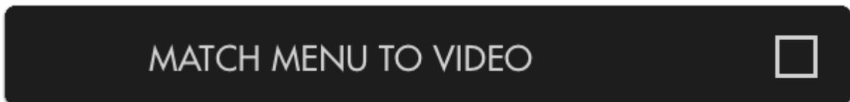
For situations with an upside-down camera - low mode on a stabilizer for example - use this option to rotate the image and not the menu.
