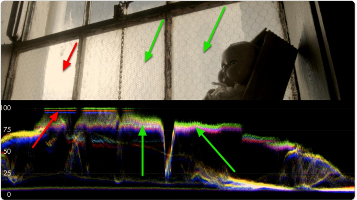
If we keep rolling exposure down (closing the aperture) we will continue seeing more 'into' the brighter details at the expense of **shadow details** which become '**crushed**' or '**clipped**' and **effectively lost** similar to overexposure.
