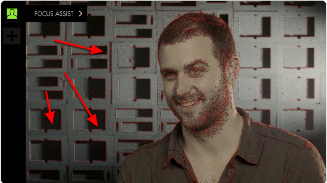
To fix this, **edit Focus Assist** by **tapping** on it when it is highlighted in the tool bar, and navigate to **Peak Threshold**.
