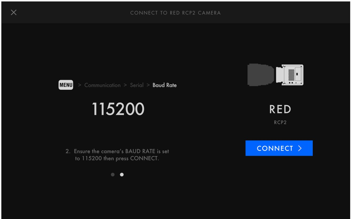
Connect your USB cable to the port on the back of your Monitor, wither directly using the Camera Control cable and USB adapter (If Applicable), below the battery plate. Tighten the locking connector into the adjacent screw for security. Connect the other end of the cable to your camera. Be sure the serial communication is enabled on the camera and that the baud rate is set to 115200.
