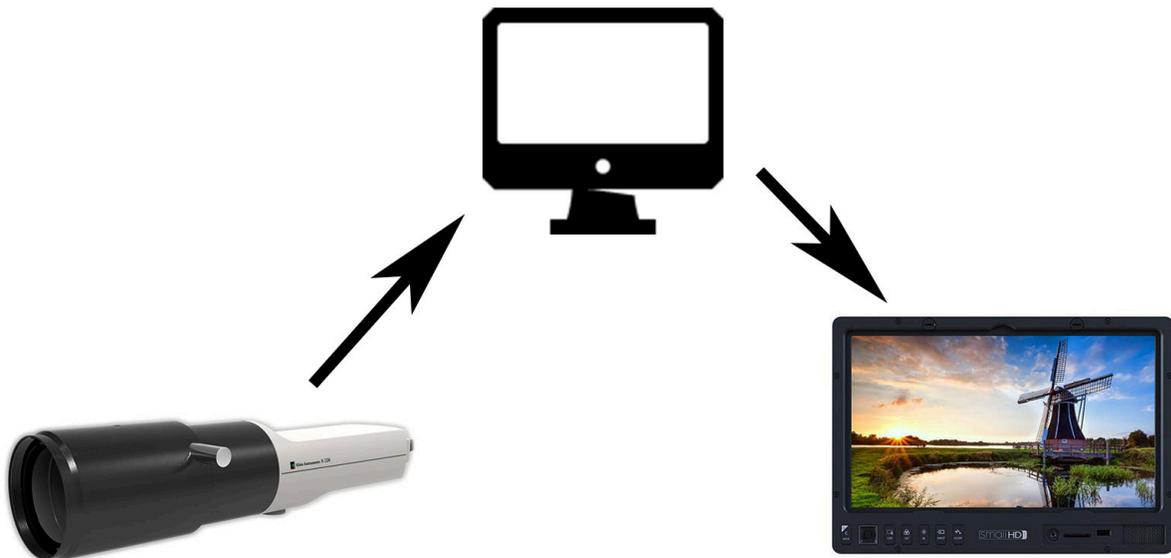
We recommend probes that can handle at least 2000 nits of brightness and 1:100000 contrast ratios (depending on your monitor Nit level, your probe should handle more). Common professional calibration probes include the [Klein Instruments K-10A](#) and Colorimetry Research CR-100. More budget probes are available on the market, you will get what you pay for in many cases.
