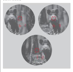
Your Leica Geovid HD-B/HD-R can also be used for continuous measurements (scan mode): Hold the main/trigger button 1 when you press it a 2nd time. After about 2.5 seconds, the device switches to scan mode and will then measure continuously. Scan mode is indicated by a change in the display:
