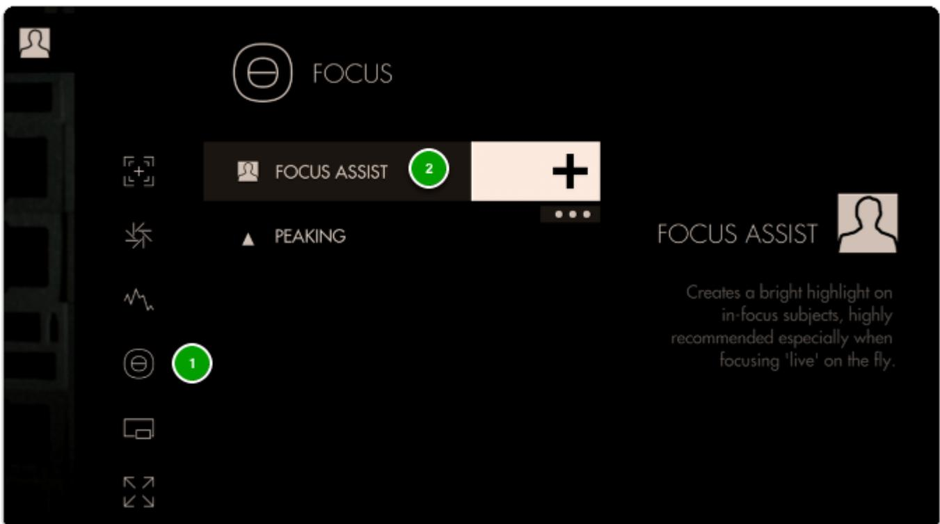
Focus Assist will paint a **highlight** around areas it determines to be in focus based on small/harsh changes in contrast.
