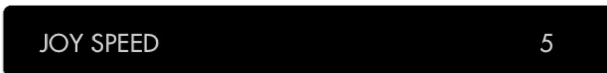
Adjusts the speed at which the color picker crosshair will glide across the screen when moved with a joystick.
