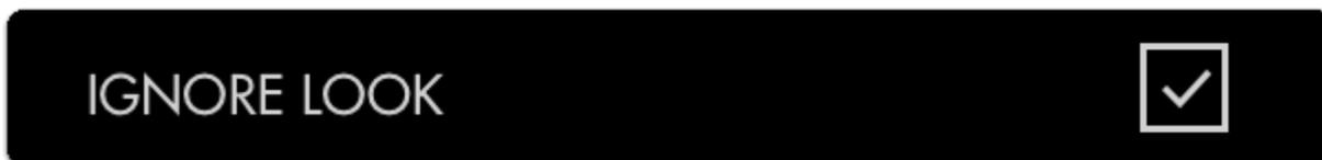
Because monitoring with a Look (3D LUT) alters the image and therefore its exposure, it can be useful to ignore its effects on exposure tools. This means you can monitor with any graded Look while using the Histogram to set up your camera to be exposed properly for any other grading possibilities in post because it's working off the camera's original ungraded image.
