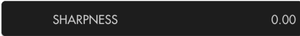
Adjusts the intensity of edge detection. See [Peaking](#) for a more user-friendly version of this.
