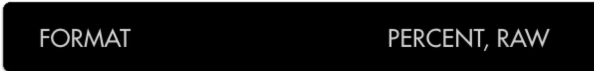
Choose how you wish to display brightness ranges - via percentage or raw image value which will change depending on bit depth (8-bit is 0-255, 10-bit is 0-1023, etc).
