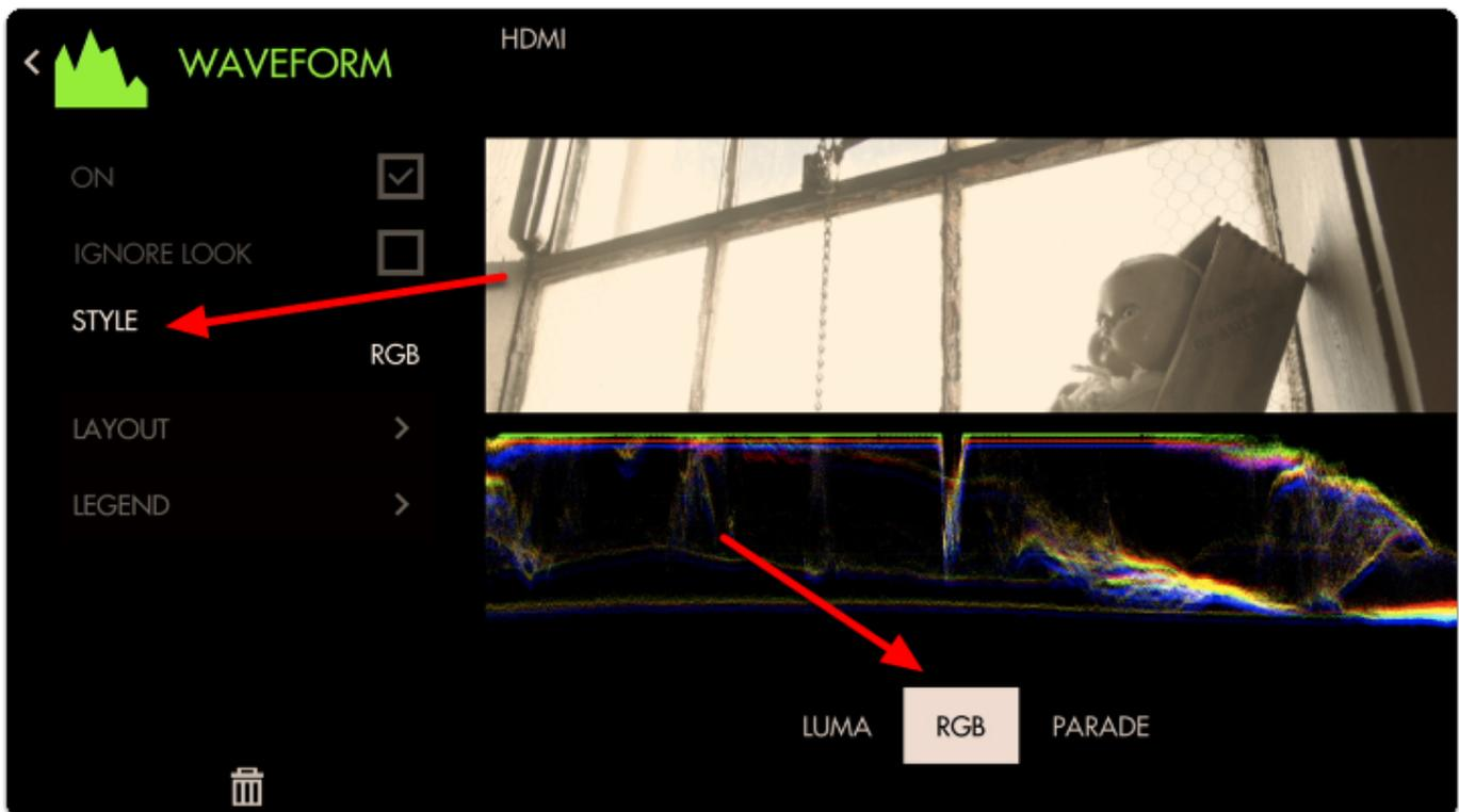
Back out of the Edit Tool menu to observe the waveform in action and to accurately expose your footage.
