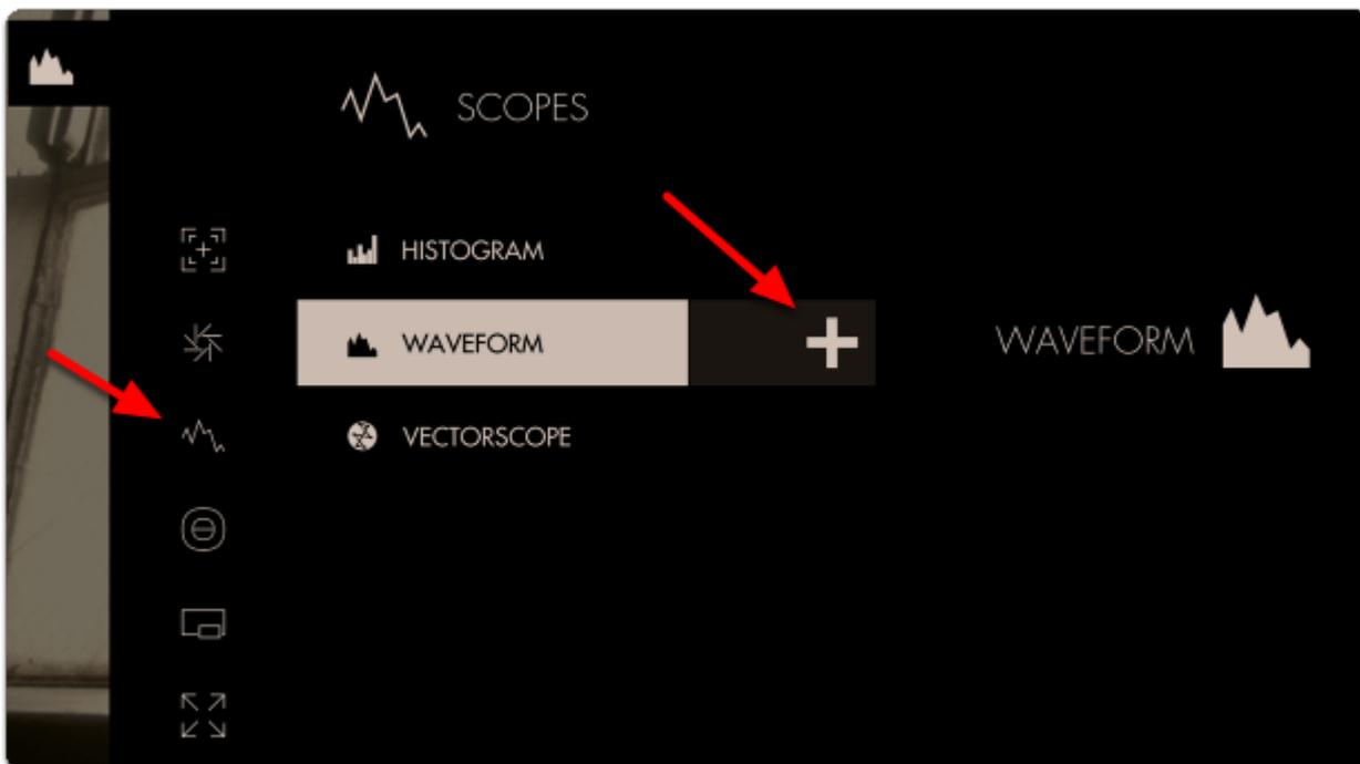
Once added you can edit the settings by navigating right when 'Waveform' is highlighted.
