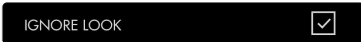
Allows you to apply a Look (3D LUT) to your footage while monitoring a waveform that is not affected by the Look. This lets you make exposure decisions based on the signal coming from the monitor for ideal flexibility in post-production.
