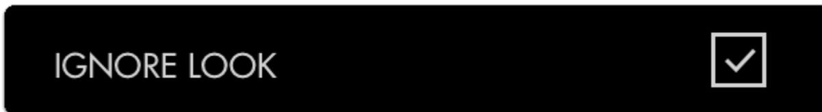
When using a Look (3D LUT) file, you may want to enable this feature which applies the zebra tool to the **original picture** coming into the monitor and **ignores the applied 3D LUT** which would alter the points at which the tool would activate. This is important because it allows you to adjust for the original shot, giving you the most flexibility in post.
