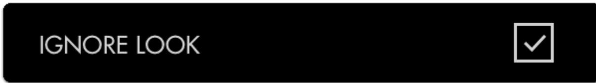
Allows Exposure Assist to work on the signal directly from the camera even if you have a Look (3D LUT) applied which would otherwise affect the results on the scale. Uncheck if you wish to monitor exposure values AFTER a look has been applied to see what effect it may bring to the final image.
