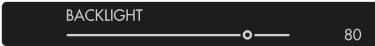
Adjusts the actual output of the backlight or in the case of OLED adjusts the maximum pixel brightness.
