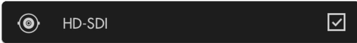
This option will send HD-SDI 'downstream' via the 'HDMI OUT' port on the monitor.
