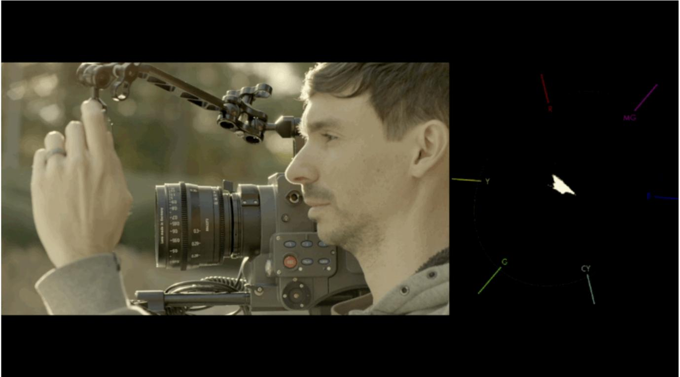
Though generally not considered as 'mission critical' during shooting as exposure scopes such as Waveform & Histogram, the Vectorscope plots the chromacity, or the hue + saturation of your image onto a color wheel so you can help gauge complimentary color, ensure skin tones are being colorized properly, to visualize how overall scene color is being placed, and where potential adjustments may need to be made in general.
