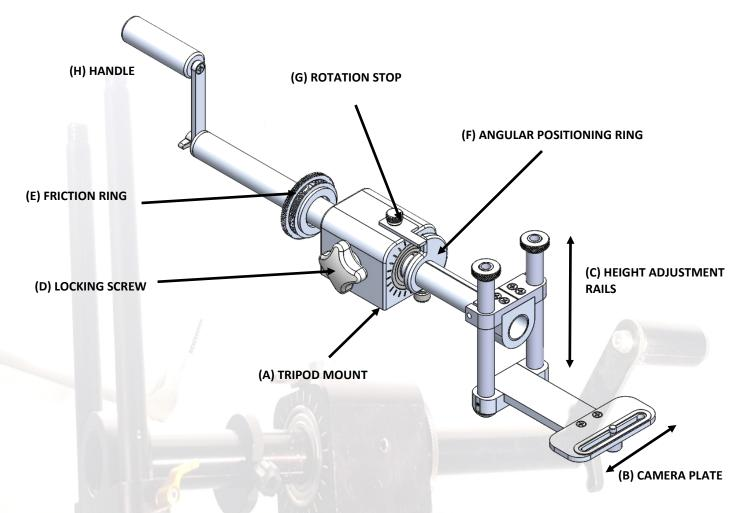
**Step 1**: Mount the DAR 100 on a tripod using one of the treaded holes at the bottom of the TRIPOD MOUNT (A)
