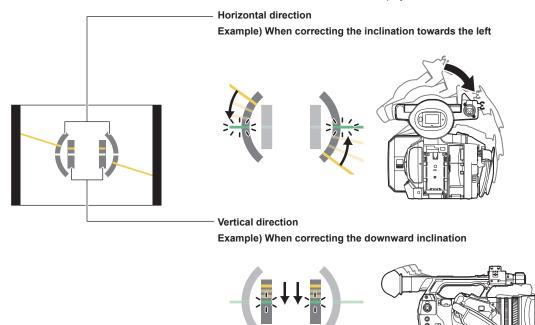
Orange lines will be displayed when inclined. Orange lines will be changed to green lines when there is almost no inclination. Inclinations will be displayed up to approximately ±45° in the horizontal direction, and up to ±30° in the vertical direction.
