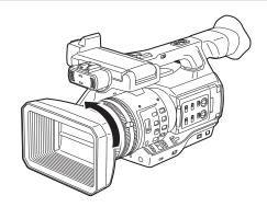
1 Rotate the lens hood counter-clockwise.
