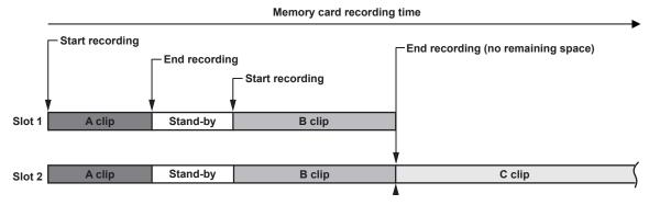
Selecting [ON] in the main menu  $\rightarrow$  [RECORDING SETUP]  $\rightarrow$  [SIMUL REC] will set the camera to simultaneous recording mode.
