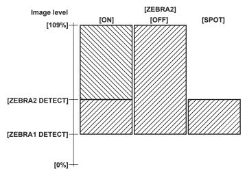
To display the zebra patterns in the video of the monitor output terminal ( $\langle GENLOCK\ IN/VIDEO\ OUT \rangle$ ), set in the main menu  $\rightarrow$  [OUTPUT SEL]  $\rightarrow$  [VIDEO OUT ZEBRA].
