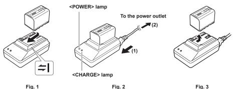
1 Place the battery horizontally along the =| mark in the battery charger and slide it in. (Fig. 1)
