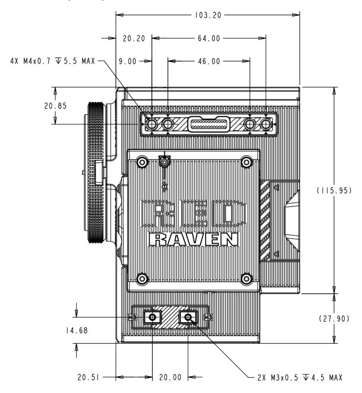
Figure: RAVEN Side View (Right)
