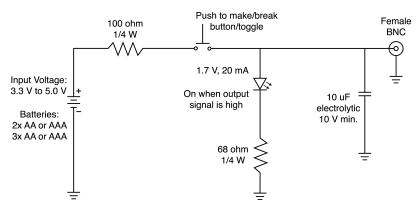
Figure: Trigger Button Circuit Diagram
