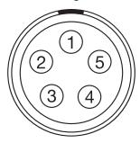
Figure: Front Face of Timecode (LEMO EAG.0B.305.CLN) Connector (Looking at the Camera)
