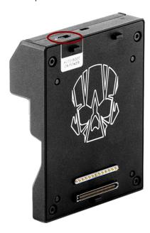
Figure: Auto Boot on Power Switch
