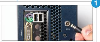
Connect the TriCaster power supply cable to the DC IN port on the rear panel and plug into an electrical outlet or external power source
