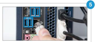
Plug an Ethernet cable into the TriCaster Ethernet port and connect to an active local network
