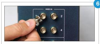
Connect an appropriate SDI accessory cable to camera and plug in using VIDEO IN port 1; repeat using ports 2-4 for additional cameras
