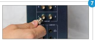
Connect the cable for SDI output to VIDEO OUT port 1; repeat using port 2 for additional SDI output, as needed
