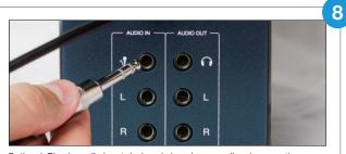
Optional: Plug in audio input devices (microphone, audio mixer, or other sound source) using the appropriate 1/4" AUDIO IN jacks
