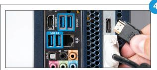
Optional: Connect the cable for Multiview monitor to the HDMI port on the right
