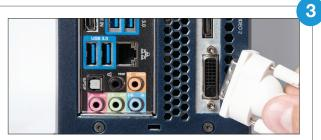
Connect the cable for User Interface monitor to the DVI port on the right
