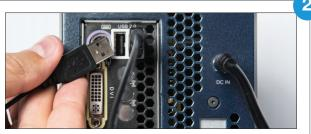
Connect the keyboard and mouse using USB ports
