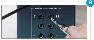
Optional: Plug in audio output devices (headphones, speakers, or sound system) using the appropriate 1/4" AUDIO OUT jacks
