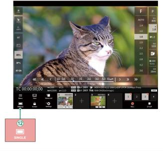
(12) A 4-screen display button has been added. If this button is pressed, the screen display is divided into four parts to check the live views of multiple cameras at the same time.
