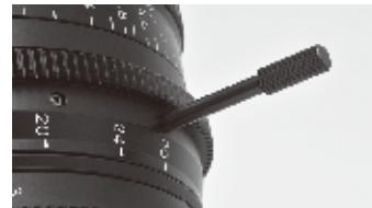
Use care when screwing on the focus/zoom pin. The pin must be aligned straight with the corresponding holes. If not, the threaded hole could get stripped or damaged.
