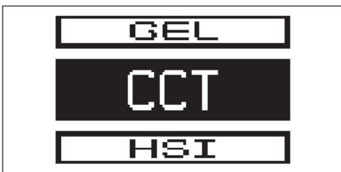
2.2.1 Short press INT wheel to select CCT mode to adjust color temperature (2000K~10000K).
