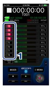
1. Tap the track selection buttons on the HOME screen for the inputs to record.
