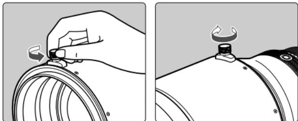
The dedicated Lens Hood ET-155 helps to prevent stray light from entering the lens and protects the front of the lens from rain, snow or dust.
