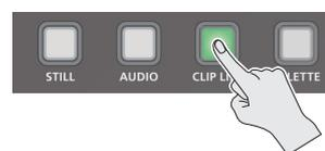
The CLIP LIST screen is shown in the lower half of the built-in display.
