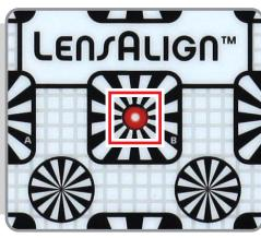
After sighting is complete, do not change the position of the test camera or LensAlign. Sighting must be checked and possibly repeated if the camera or LensAlign is moved. Be sure to set the camera to Manual or Aperture Priority exposure mode and open the aperture of the lens to its lowest *f* stop (wide open). You are now ready to capture test images.
