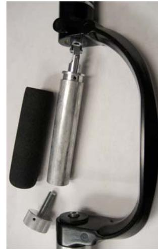
Remove knurled knob from the handle by completely unscrewing it, then remove foam grip by sliding it off the handle. Store the foam grip for later use.
