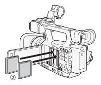
You can check the status of the CF card slots immediately by looking at the CF A/CF B access indicator. Refer to the following table.
