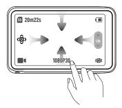
**Tap once:** tap an icon to select features such as smart gimbal mode and rotate the camera. Tap on the live view for focusing and spot metering.
