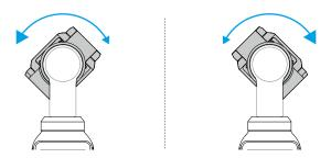
• When 180° is selected, press the 5D joystick or tap  $\bigcirc$  to enable SpinShot mode with 180°. The camera will recenter first and face upward, and then rotate 180° on the pan axis.
