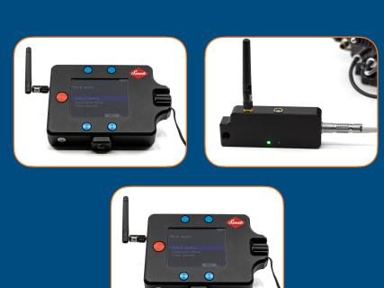
If using a direct ethernet connection for camera control, "Local" will be your only option. If using a wireless connection, press the blue button on the remote above "New." Push in to select either option.
