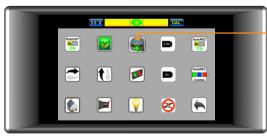
From the main menu, select Tools icon. then activate Virtual Horizon. When the horizontal bar is displayed on the top of the monitor screen, tap on CAL button.
