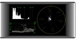
Displays available measurment tools. Histogram & Waveform can be pinned on the picture by simply touching their representation on this screen.
