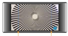
Peaking is applied to the image area located between the two vertical bars.
